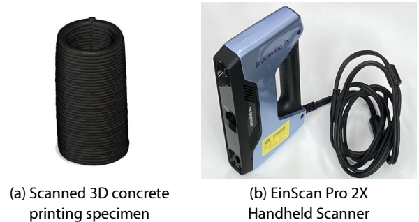
Fig. 10 Scanning 3D concrete printing specimens
