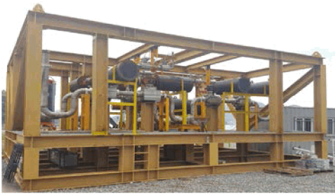
Fig. 1 Real manifold system for offshore subsea plant
