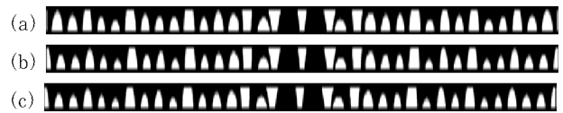
Fig. 5 Optimal configuration obtained by changing initial phase field parameter value; (a) 0.5, (b) 0.6, (c) 0.7
