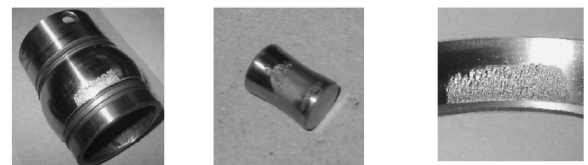
(a) Inner race (b) Roller element (c) Outer race
