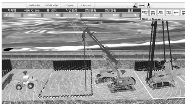
Fig. 12 Virtual excavation simulation in the vicinity of the existing rail road (Construction of lot 3-3, Honam high speed railway(KTX), Daelim)
