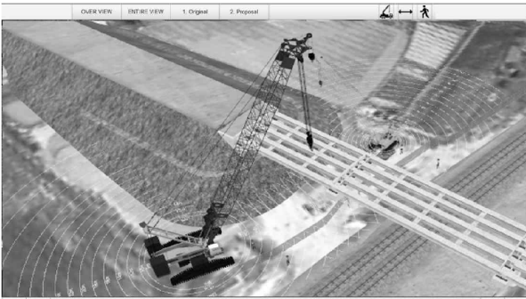
Fig. 11 Virtual election simulation of bridge beam (Construction of lot 3-1, Honam high speed railway(KTX), Dongbu corporation)
